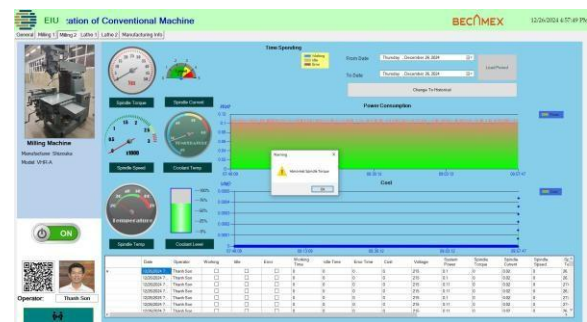
Figure 4: The user interface of the milling machine with the warning message "Abnormal Spindle Torque"
